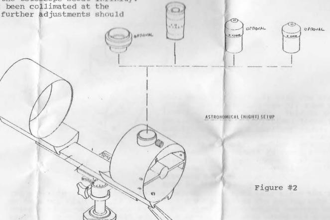
The camera adapter has two bodies. One is for eyepiece projection where the eyepiece is inserted in the housing and the other is for prime focus photography. Exchange the T-ring adapter from one housing to the other.
